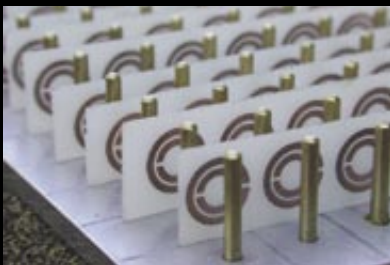
A metamaterial is made by creating an array of wires and SRRs that are smaller than the wavelength of the electromagnetic waves to be used with the material.
