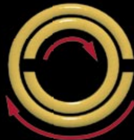
Circular currents flow in split-ring resonators (SRRs).
