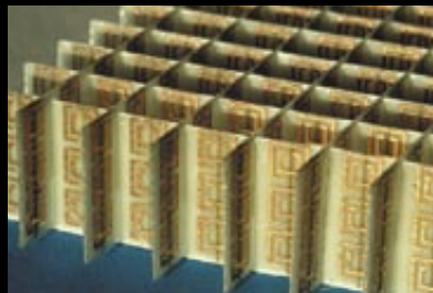
A metamaterial is made by creating an array of wires and SRRs that are smaller than the wavelength of the electromagnetic waves to be used with the material.
